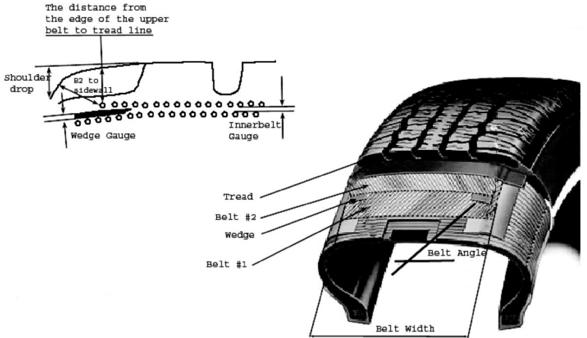
Fig. 1. Elements of radial tire.
