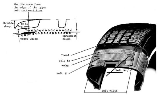
Fig. 1. Elements of radial tire.
