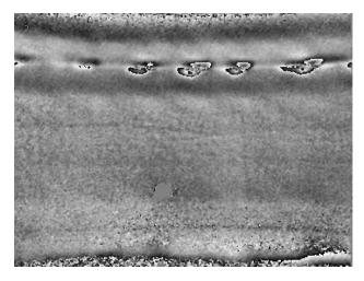
Fig. 6. Example of tire shearography.
